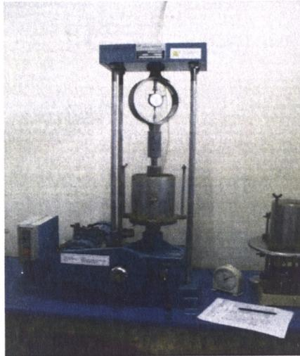
Gambar 7.25 Alat Uji CBR Laboratorium
